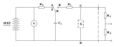
$\begin{array}{lll} \text{Note:} & C_1 = 0.01 \mu F < 10,000 V & C_1 = 1 n F \; (0.001 \mu F) \geq 10,000 V \\ & R_1 = 1 k \Omega & R_2 = 100 M \Omega & R_3 = 0.1 M \Omega & R_s = 15 M \Omega \end{array}$
